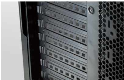
EIGHT PCI VENTED SLOT COVERS FOR BETTER FLEXIBILITY & COOLING PERFORMANCE
